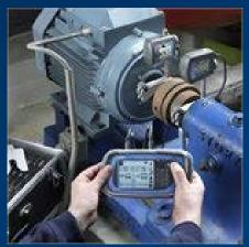
Aligning rotating equipment within recommended specifications
