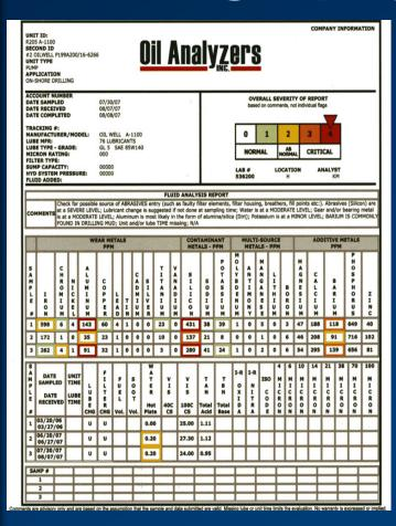
Analyzing the particles present in fluids that indicate mechanical wear
