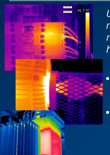
Uses infrared imaging, detecting radiation in the infrared range, to measure and visualize relative heat of objects
